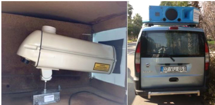
Figure 4. Automatic number plate recognition setup placed on the vehicle [3,53].
