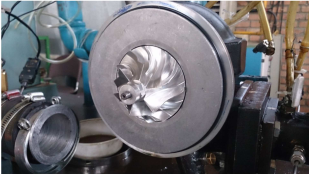
Figure 12. Modified impeller mounted on turbocharger shaft.
