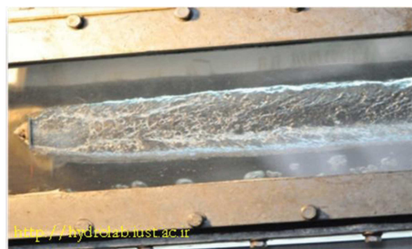
Figure 1. Ventilated supercavitation produced in hydrodynamic laboratory at Iran University of Science and Technology.
