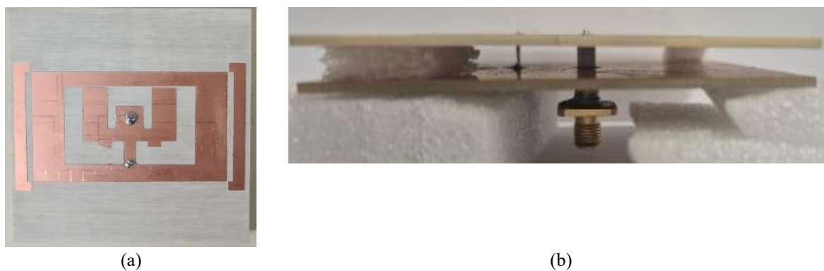
Figure 7. Fabricated dual-band antenna, (a) Radiation part (top view), (b) Grounded pin and SMA connector (side view).
