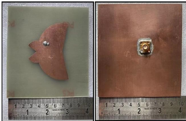
Figure 13. Photograph of the fabricated layout of the proposed tri-band antenna.
