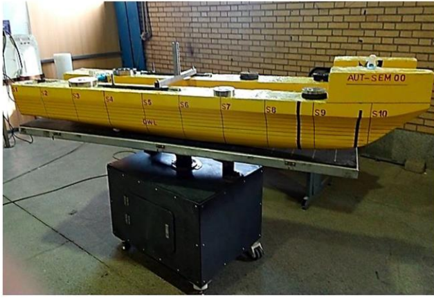
Figure 3. Measuring and setting up the moment of inertia of the model.
