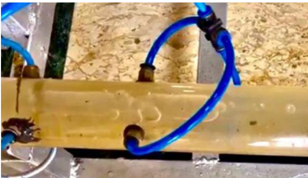
Figure 11. Real view of 3rd stage ventilation through the transparent pipe at 1400 rpm.
