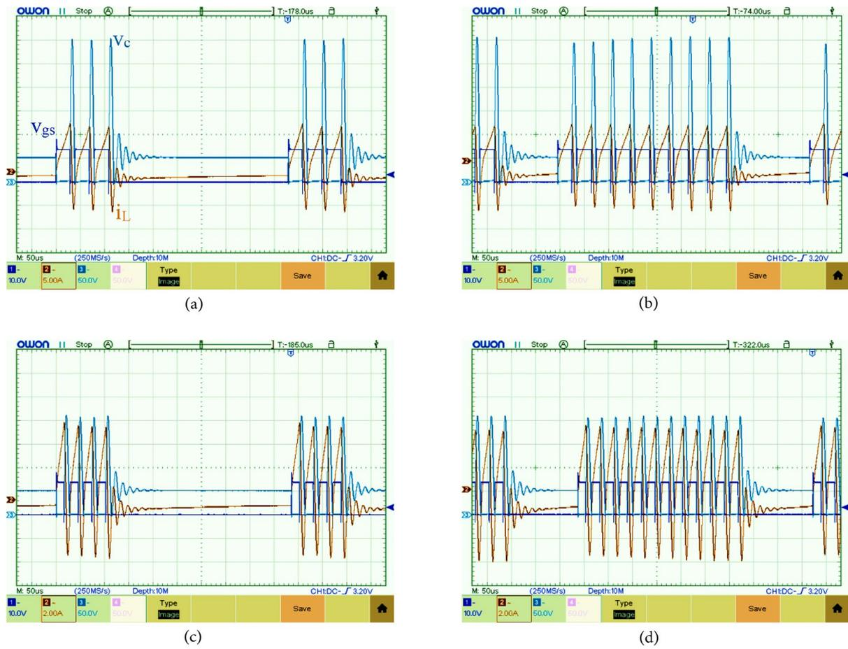
**Figure 19.** The waveforms of the gate signal, coil current and capacitor voltage at different temperature and time values of the curve in Figure 17: (a) For 50th second and 56°C; (b) for 110th second and 223°C; (c) for 124th second and 261°C; and (d) for 225th second and 251°C.
