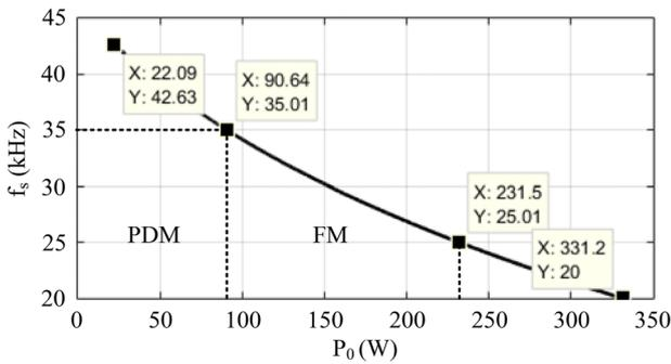
Figure 11. The power-frequency curve of the hybrid control.
