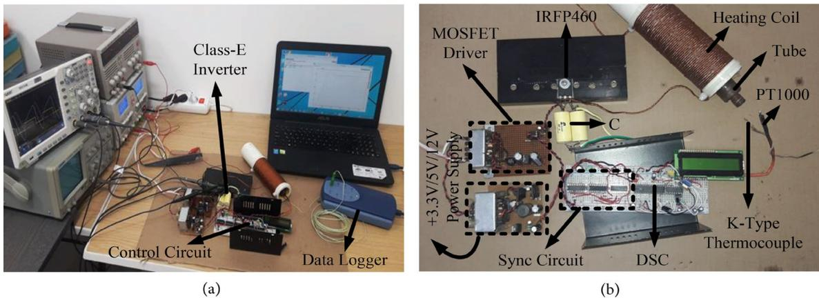
Figure 13. The induction heating system: (a) The experimental setup; and (b) the inverter and control circuit.
