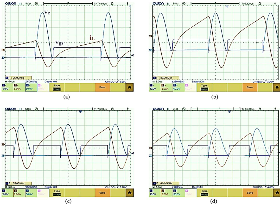
Figure 14. The gate signal of the power switch, coil current, and capacitor voltage waveforms for different frequency values: (a) 25 kHz; (b) 30 kHz; (c) 35 kHz; and (d) 40 kHz.
