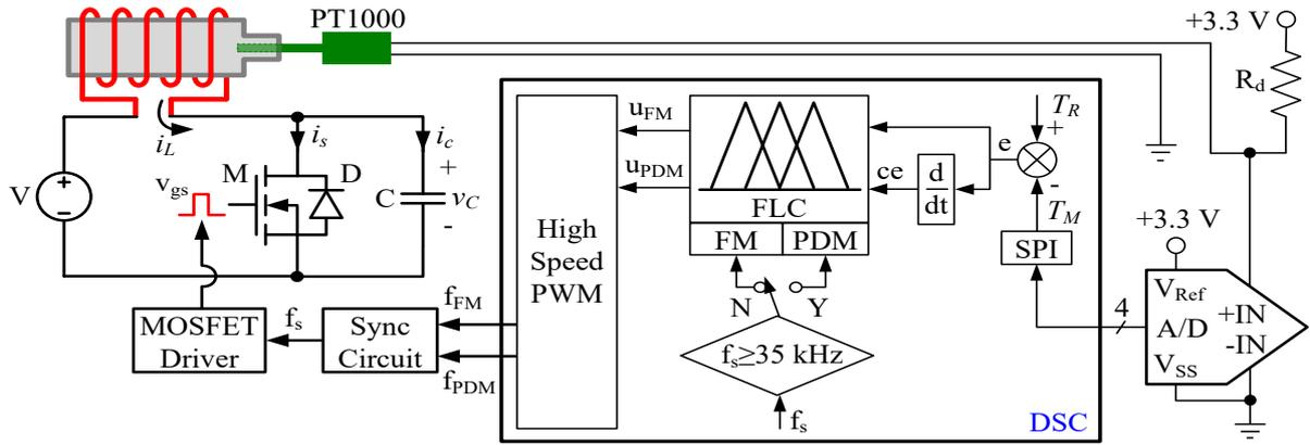
Figure 1. Induction heating system.
