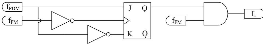
Figure 2. The synchronization circuit.
