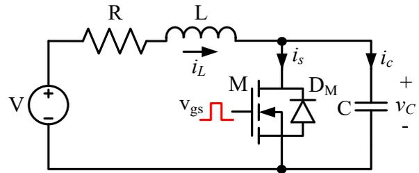
Figure 3. The equivalent circuit.
