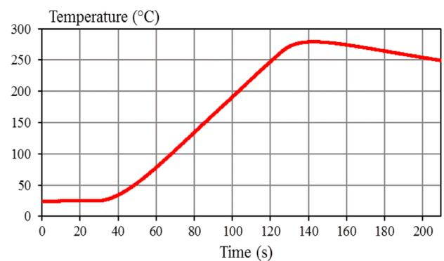
**Figure 16.** Temperature-time graph of the workpiece for the fixed operating frequency of 25 kHz.
