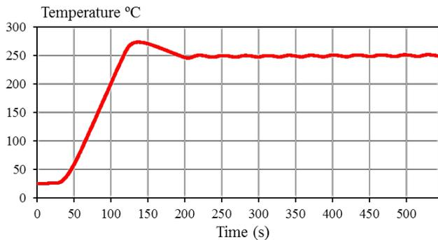
**Figure 18.** The response of the closed loop system.
