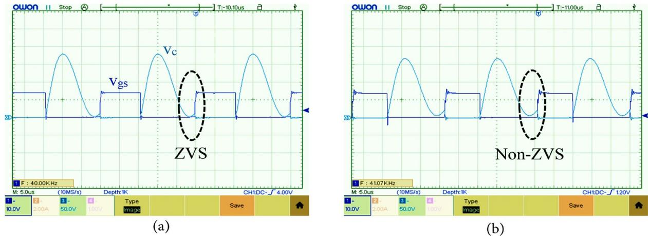
**Figure 15.** The states of ZVS for the different frequencies: (a) 40 kHz; and (b) 41.07 kHz.
