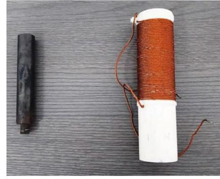
Figure 7. The tube and heating coil.
