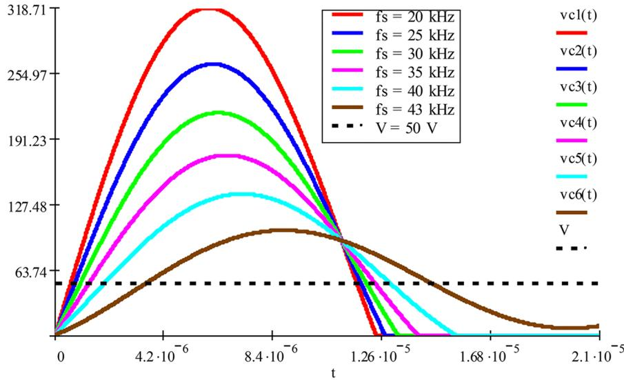
Figure 10. Variation of the capacitor voltage with the frequency for Mode 2.
