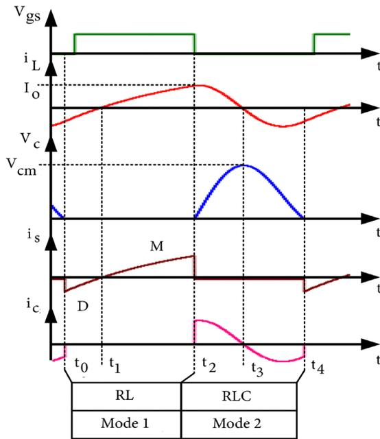
Figure 4. The waveforms of the inverter.
