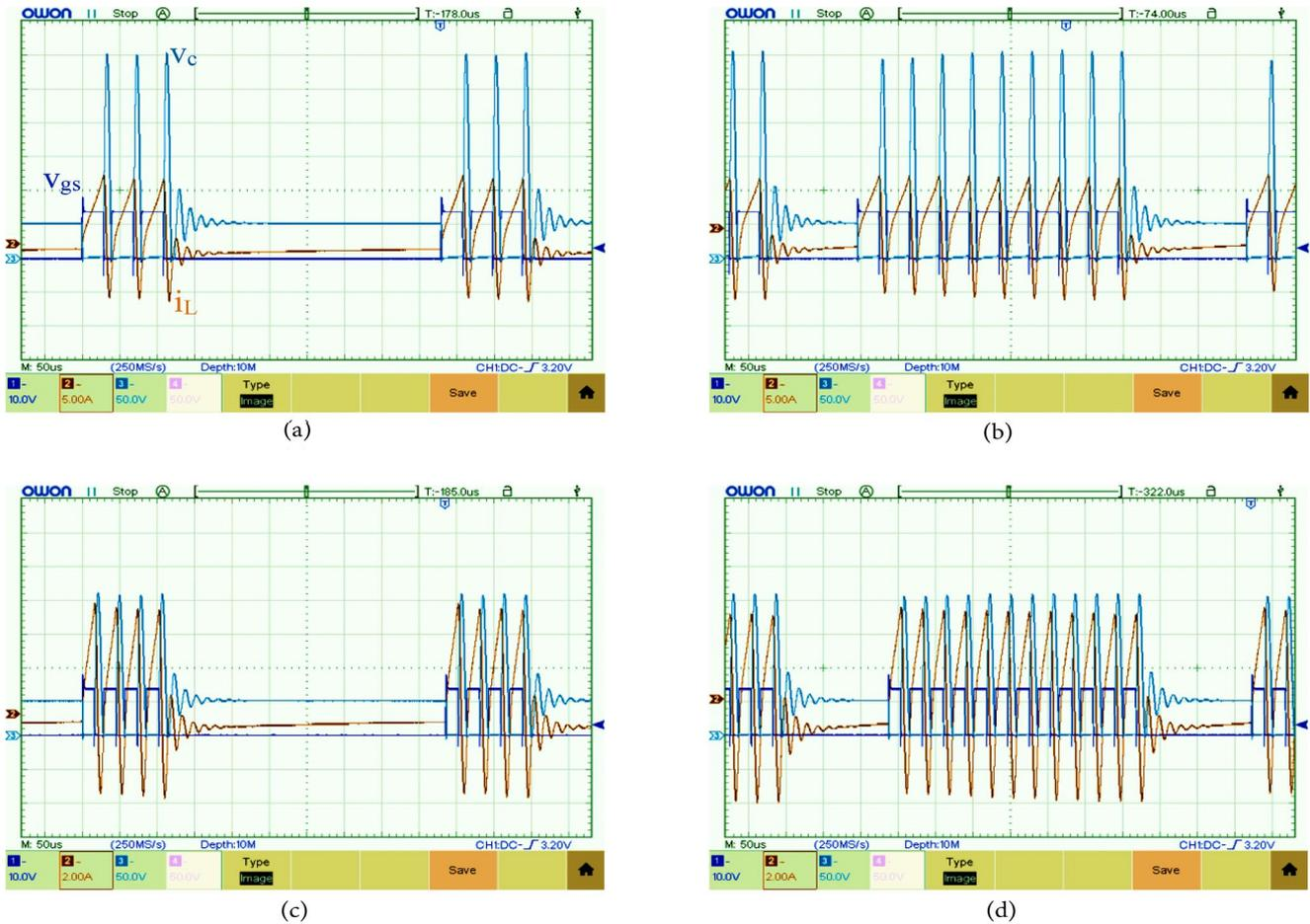
**Figure 17.** The gate signal, coil current, and capacitor voltage waveforms of the PDM controlled inverter: (a)  $f_s=25$  kHz and  $D=25\%$ ; (b)  $f_s=25$  kHz and  $D=75\%$ ; (c)  $f_s=35$  kHz and  $D=2\%$ ; and (d)  $f_s=35$  kHz and  $D=75\%$ .
