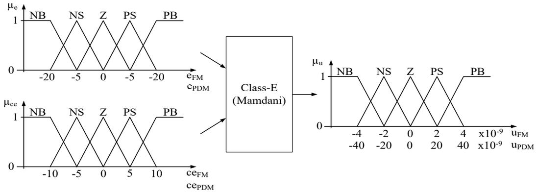
Figure 12. Membership functions of FM-PDM-based FLC.
