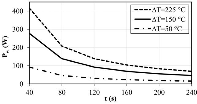
Figure 6. The power-time graph for different temperature changes.
