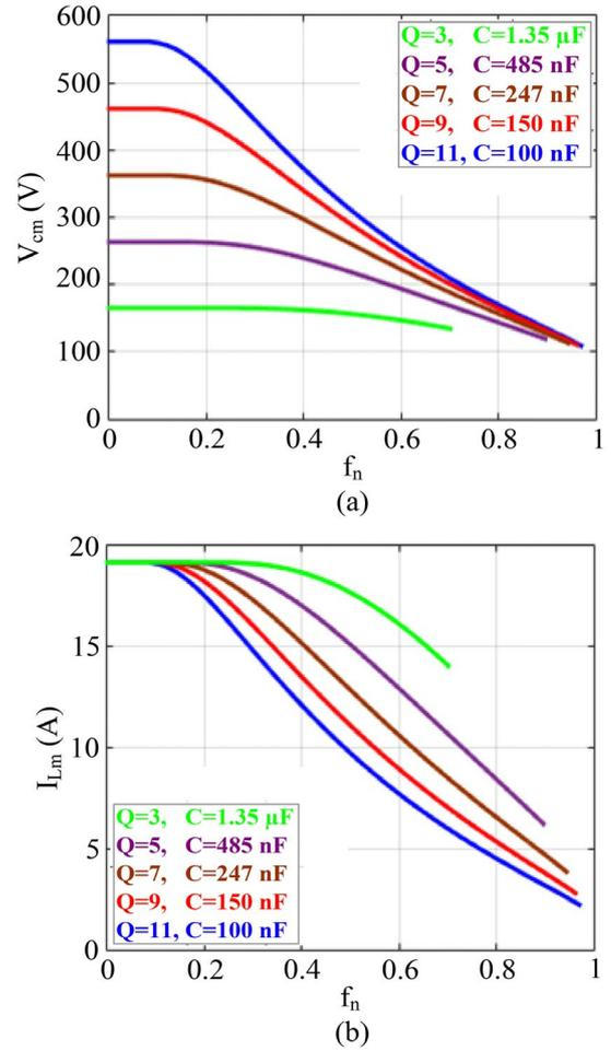
Figure 8.  $f_n-V_{cm}$  and  $f_n-I_{Lm}$  curves for different  $Q$  value, (a)  $f_n-V_{cm}$ , and (b)  $f_n-I_{Lm}$ .
