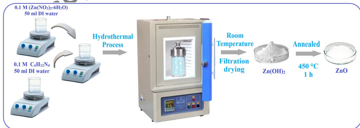
Figure 1. Diagram of ZnO particle production process and experimental mechanism.
