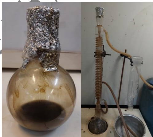
Fig. 8. Schematic representation of the apparatus used for asphaltene extraction from crude oil
