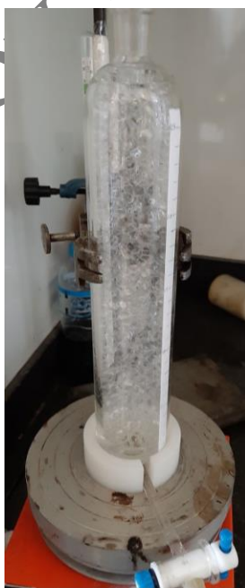
Fig. 7. The foam formed in the medium-pressure foam chamber
