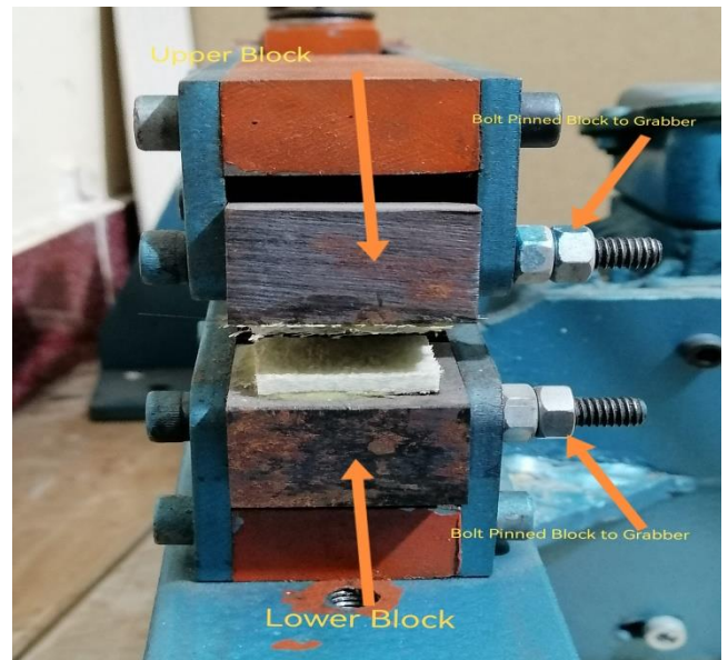
Figure 2 Specimen loaded to machine
