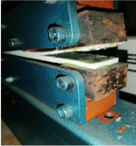
Figure 6 opening initial crack for the specimen
