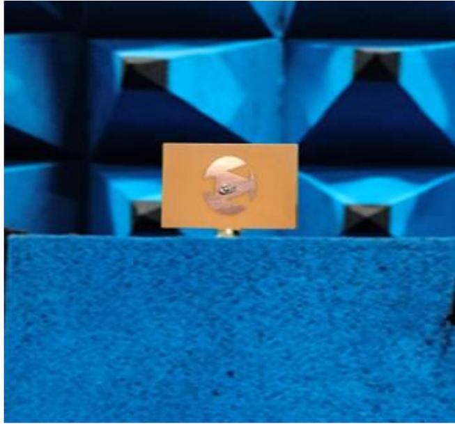
Fig.17. Presents the far field pattern measurement in an anechoic chamber.
