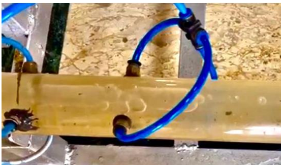
Fig. 11. Real view of 3 rd stage ventilation through the transparent pipe at 1400 rpm.
