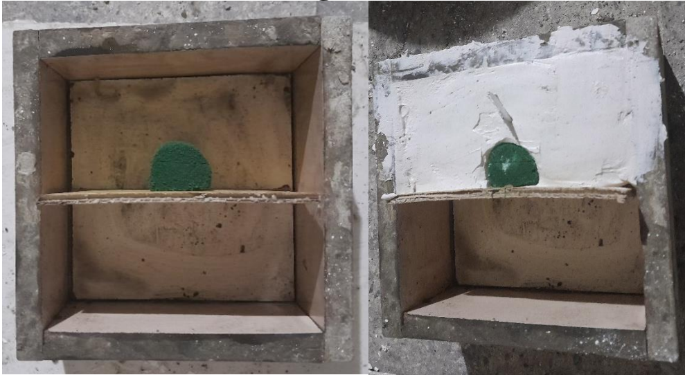
Fig. 1. Custom-designed wooden containers used for creating concrete-gypsum layers
