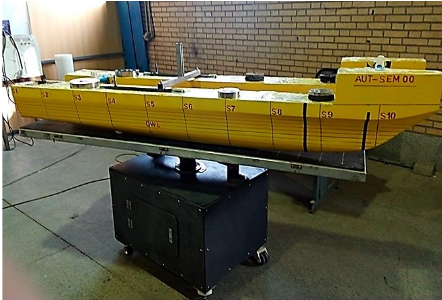
Figure 3: Measuring and setting up the moment of inertia of the model.
