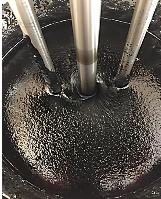
Figure 3. A sample of bitumen in additive mixing
