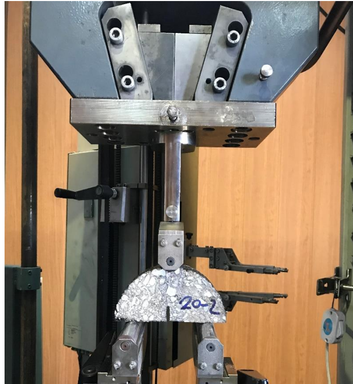
Figure 5. UTM device for static loading of samples
