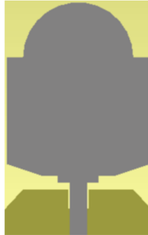
(b) Antenna-2 with UWB bandwidth
