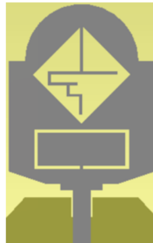
(e) Antenna-5 with dual notch band (n78, n77)
