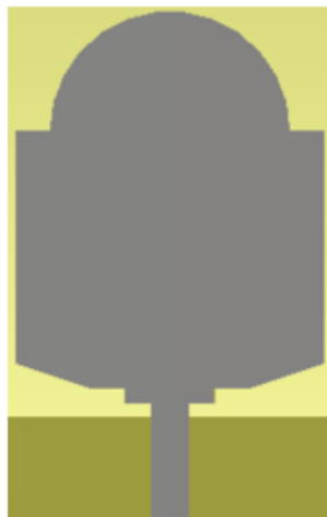
(a) Antenna-1 with partial UWB bandwidth
