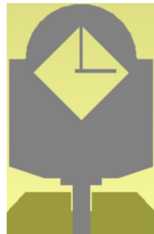
(c) Antenna-3 with single notch band (n46)
