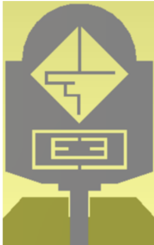
(f) Antenna-6 with triple notch band
