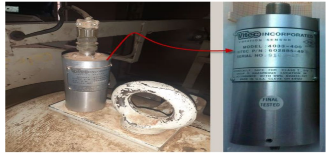
Figure 5. Position of the vibration sensor.
