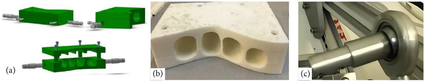
Figure 2. (a) The CAD model of digit supporters and the side shafts, (b) real model of the finger cover and (c) the real model of side shaft.
