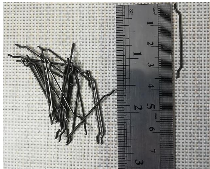
Figure 1. Steel fibers used in this research
