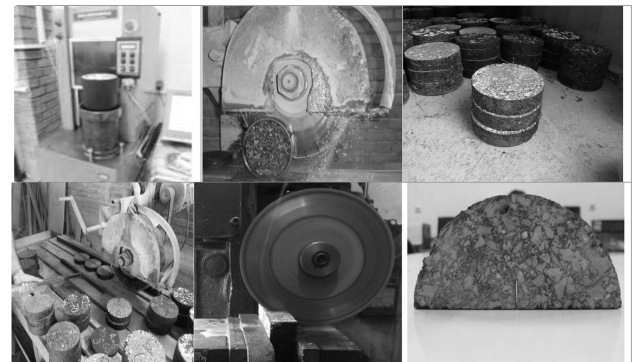
Figure 2. Some of the steps for preparing the SCB test specimens.
