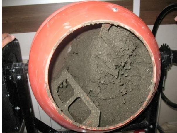
Figure 1. Drum strengthened by plate used for UHPFRC mixing in Tabriz (Iran)
