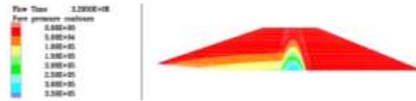
Figure13. Pore water pressure of the dam (in the end of first impounding)
