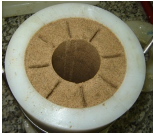
Figure 3. Removal of intact cemented HCA specimen from modified molds
