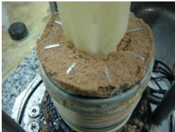
Figure 4. Failure of cemented HCA specimens under loading conditions of \alpha=45^\circ and \alpha=67.5^\circ
