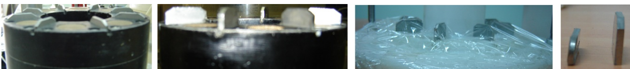
Figure 5. New taller HCA blades compared with the initial blades
