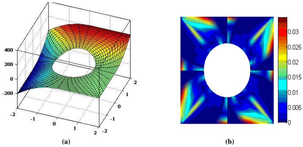
Figure 13. (a) Temperature distribution on square plate with circular hole at  $t=0$ ,
