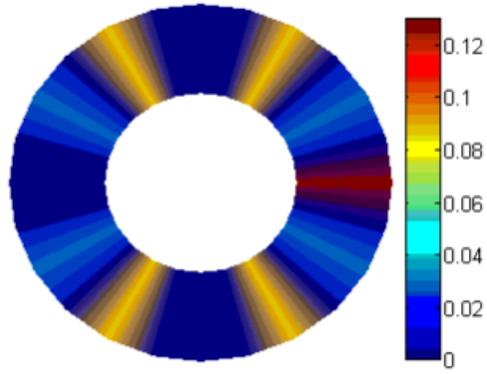
**Figure 7. Error distribution of approximated temperature at  $t=0$**
