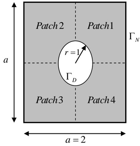
Figure 12. Square plate with circular hole in center
