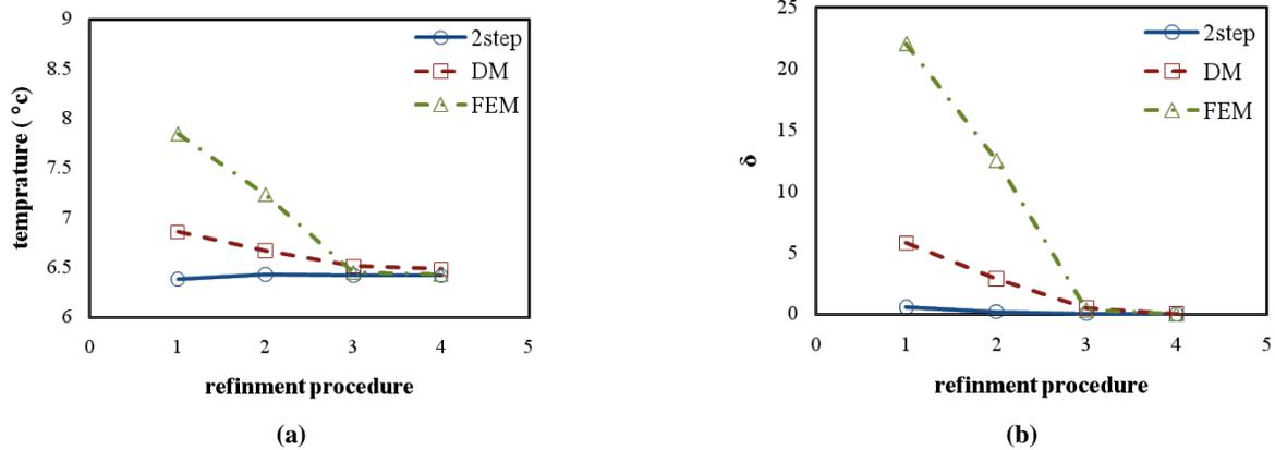
Figure 15. Convergence procedure of two-step, direct and finite element methods for example 2
