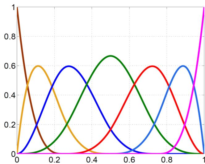
**Figure 1.** Cubic basis functions for an open knot vector  $\Xi = \{0, 0, 0, 0, 0.25, 0.5, 0.75, 1, 1, 1, 1\}$
