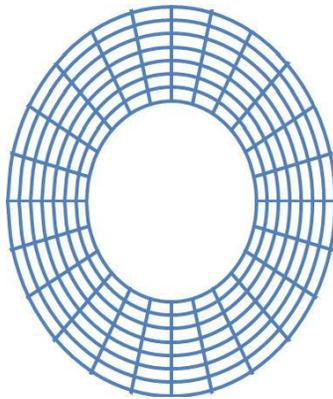
**Figure 8. Final mesh of annulus disk problem with 360 elements in IGA**
