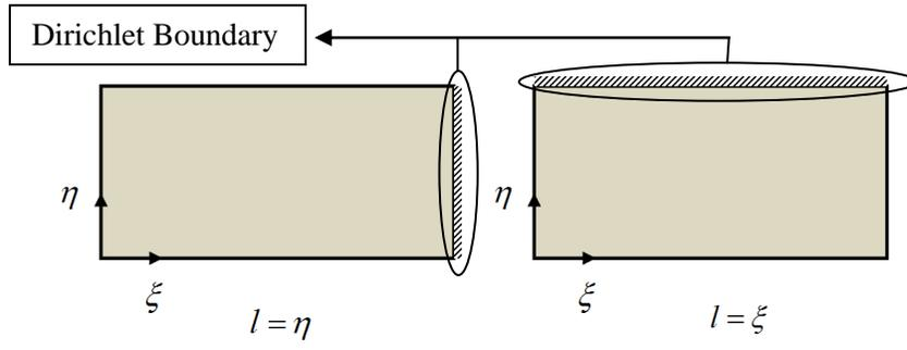
Figure 3. Direction of Dirichlet boundaries in parametric space
