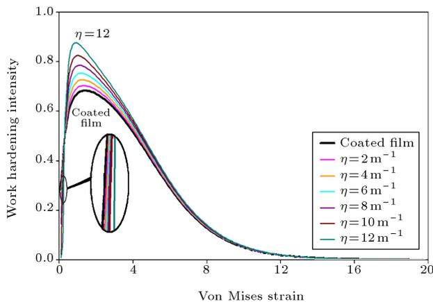
**Figure 3.** Work hardening intensity of specimens with different  $\eta$  values versus strain.
