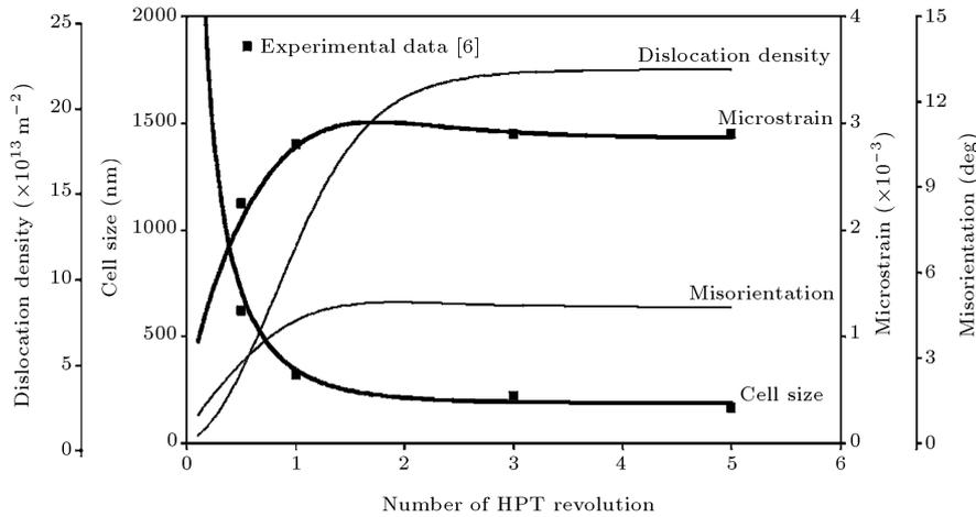
**Figure 1.** The evolutions of microstructural parameters of nickel during HPT process [6].
