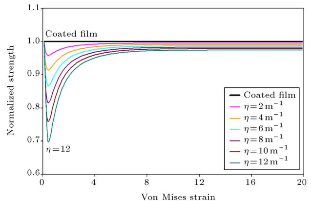
**Figure 2.** Normalized strength of specimens with different  $\eta$  values versus strain (normalized coordinate is defined in the text).
