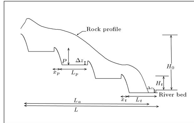
**Figure 1.** Longitudinal section of cascade of falls.
