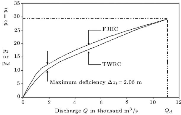
**Figure 2.** TWRC and FJHC for terminal fall - Tehri dam spillway.
