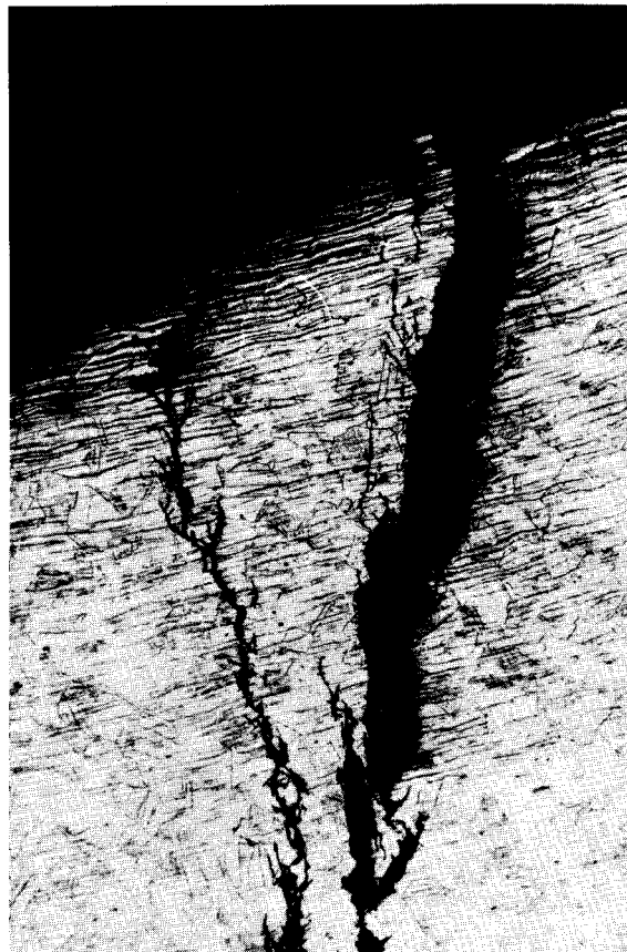
Figure 8. The produced cracks in 2500 g/lit MgCl_2 solution at pH = 3.3 ( \times 160 ).
