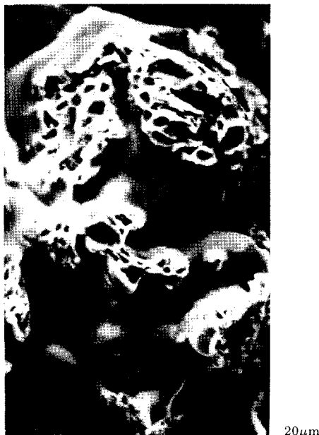
Figure 7. Fracture surfaces of Fe-1.5 Mo-0.7% C steel sintered 60 mins at 1120^\circ\text{C} , density is 6.8 \text{ g/cm}^3 , illustration of large microplasticity at sintered necks.
