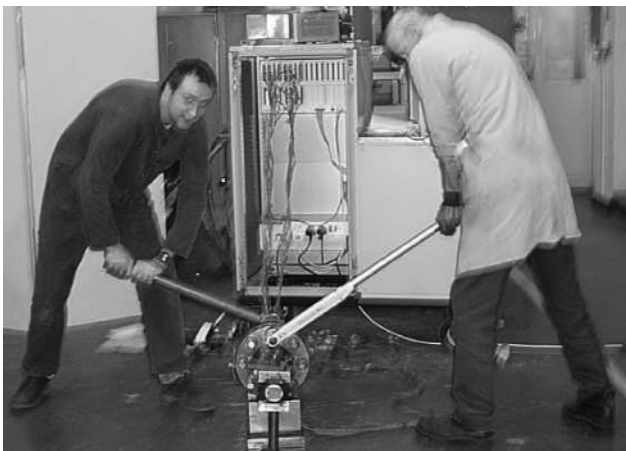
Figure 6. Arrangement for gasketed flange joint assembly.
