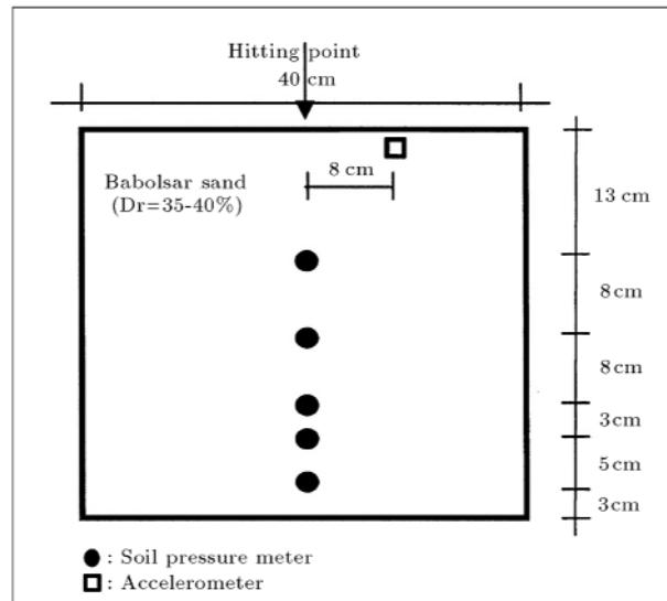
Figure 2. Typical section of the physical models and location of deployed sensors.
