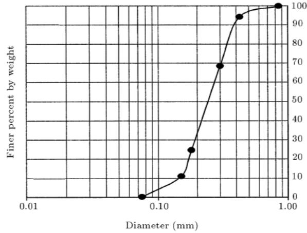
Figure 1. Grain size distribution of Babolsar Sand used for the physical models.
