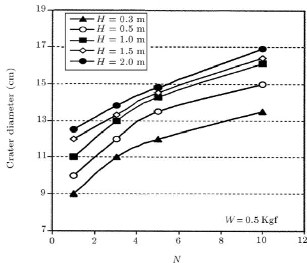
**Figure 8.** Typical measured crater diameter for 0.5 Kgf tamper, dropped from various heights.
