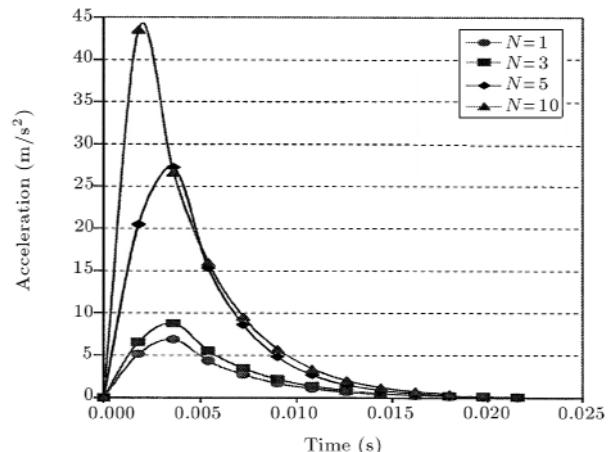
**Figure 4.** Typical recorded acceleration time histories at model surface (8 cm away from hitting point).
