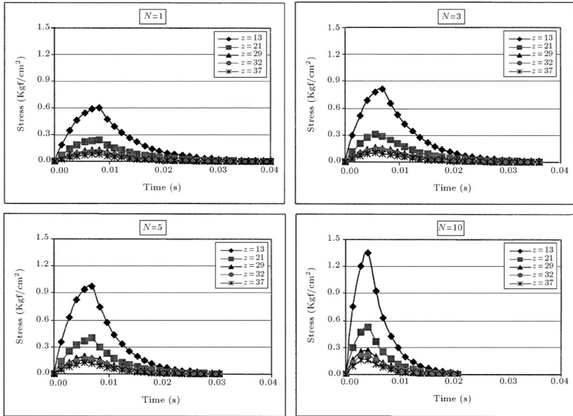
**Figure 3.** Typical recorded vertical stress time histories for 1 Kgf tamper dropped from 1m height.
