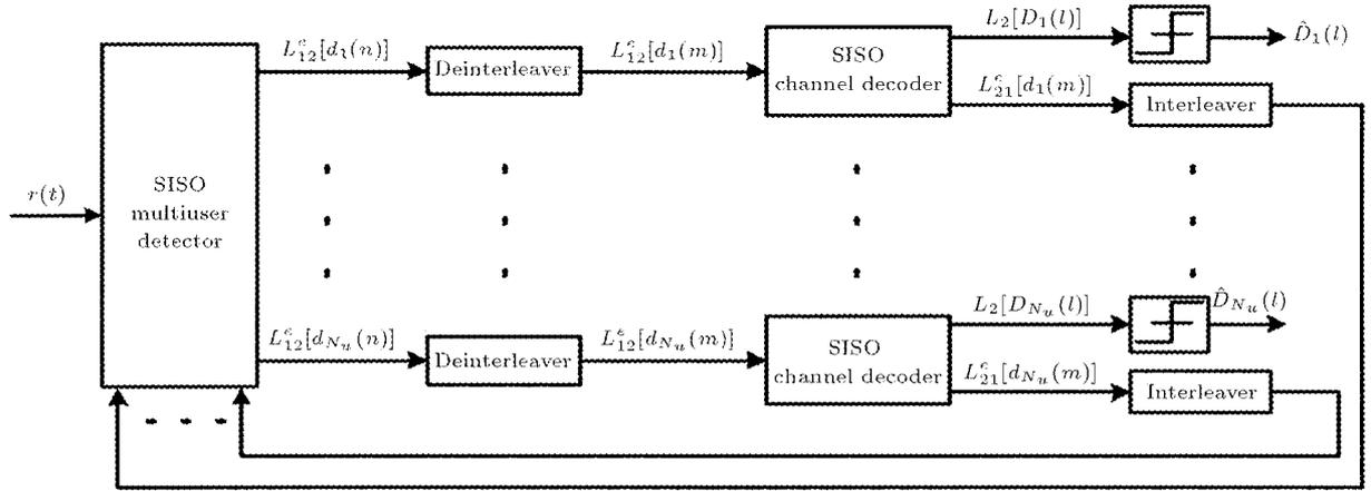
Figure 3. The block diagram of the iterative receiver.
