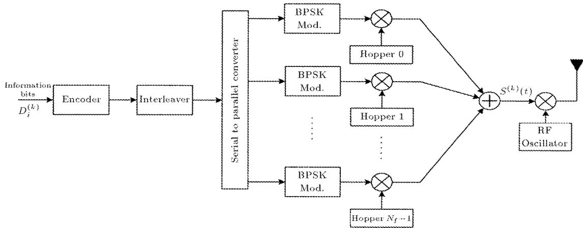
Figure 2. The block diagram of the coded MC-FH systems.
