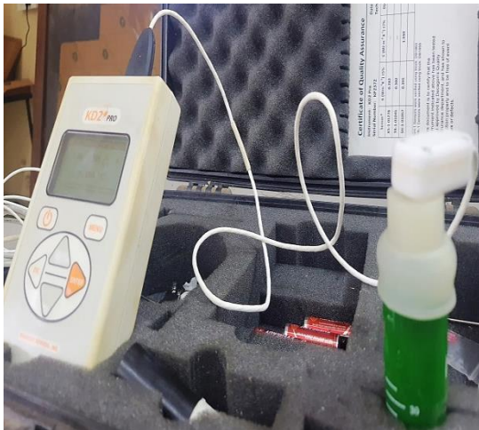
Figure 5. (a) KD2 Pro thermal analyser (b) Thermal conductivity of nanofluids
