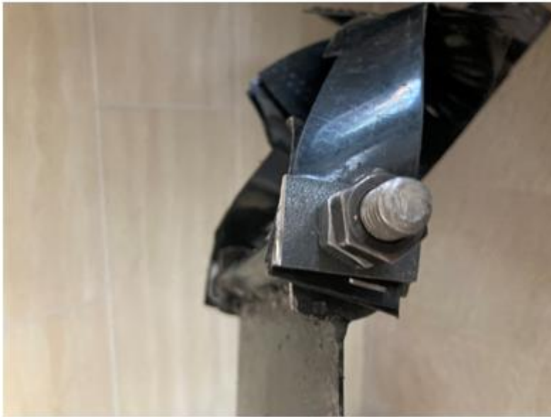
Fig. 4. Clamp designed for geocell-hydraulic jack attachment: (a) geocell attachment to clamp; (b) vertical plates
