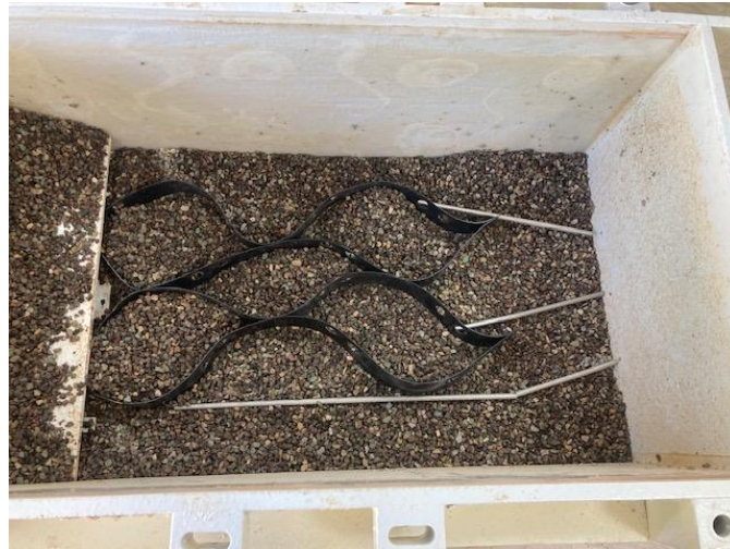
Fig. 3. Geocell placed on the lower half of soil sample
