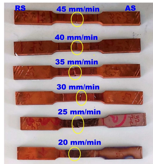
Figure 5. Photographs of the fractured tensile specimen of the CDA 101 Cu alloy joints with their exact location of fracture being highlighted.
