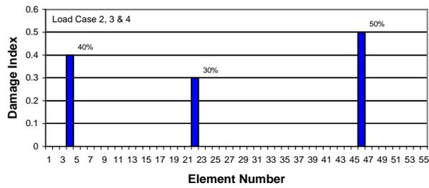
**Fig. 6.** Predicted damages for case3 using the different combination of load cases.
