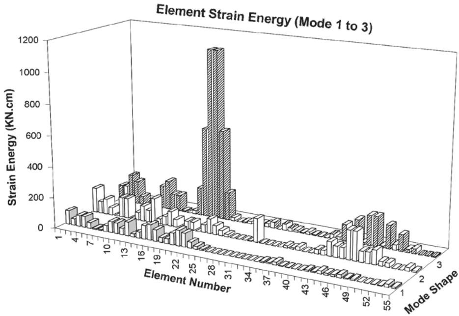
Fig. 9. Elemental strain energies of the undamaged structure due to the first three mode shapes.
