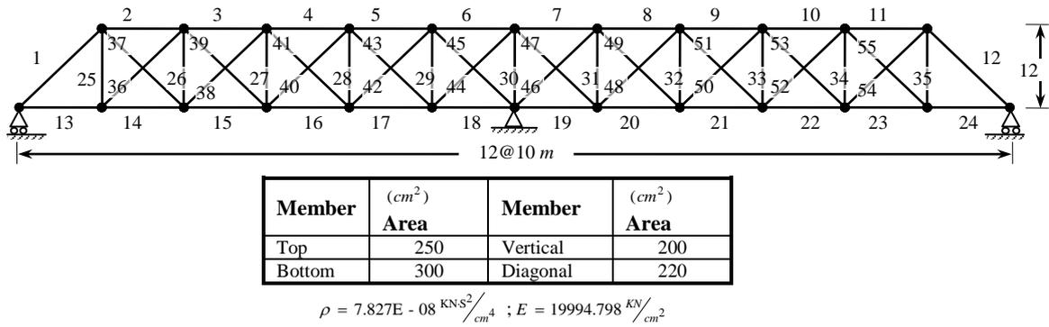
Fig. 1. Cross-sectional properties and the layout of bridge truss.
