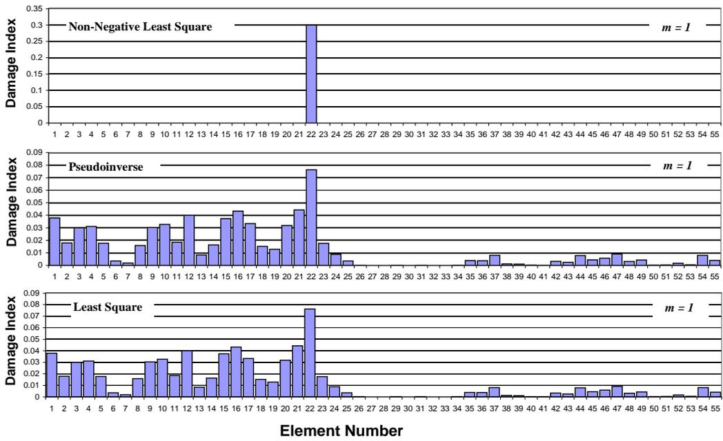
Fig. 10. Predicted damages for case1 using the first mode shape.
