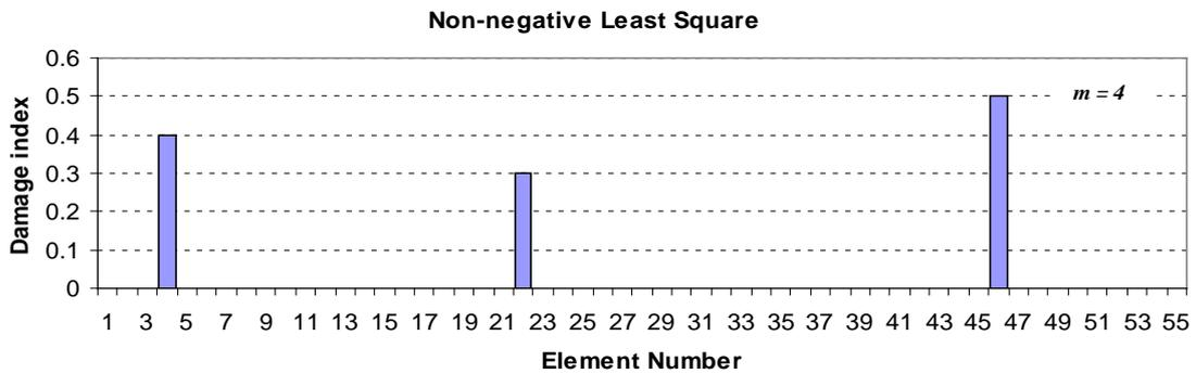
Fig. 12. Predicted damages for case3 using the first four mode shapes.
