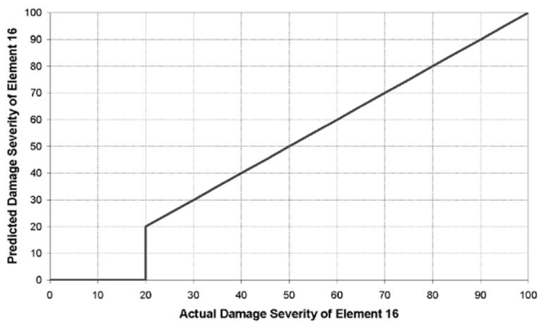
**Fig. 7.** Predicted damage for element 16 with different damage severity from static response.
