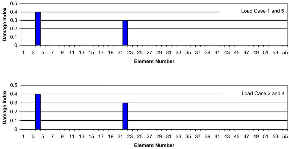
**Fig. 5.** Predicted damages for case2, when two load cases are used simultaneously.
