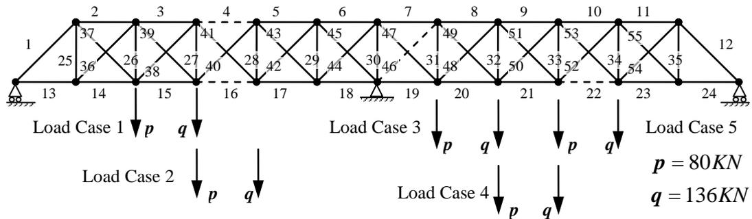
Fig. 2. Damaged members and load cases of bridge truss.
