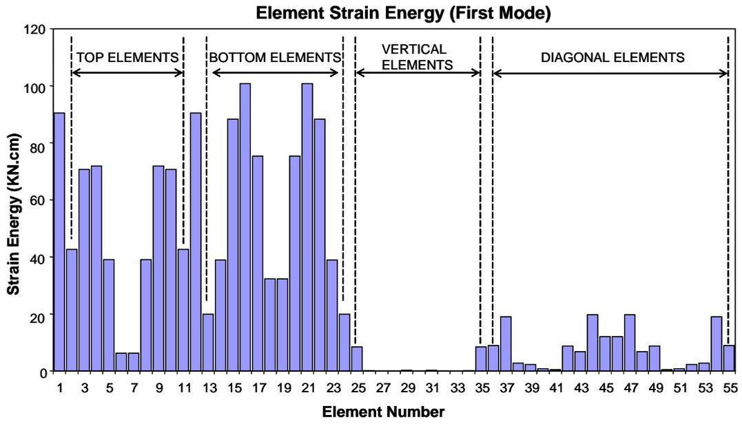
Fig. 8. Elemental strain energies of the undamaged structure due to the first mode shape.
