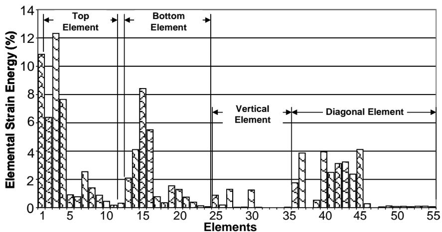
Fig. 3. Elemental strain energies of undamaged bridge truss due to load case 1.
