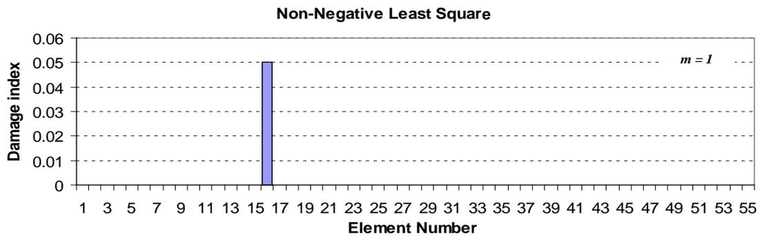
**Fig. 13.** Predicted damages for case4 using the first mode shape.
