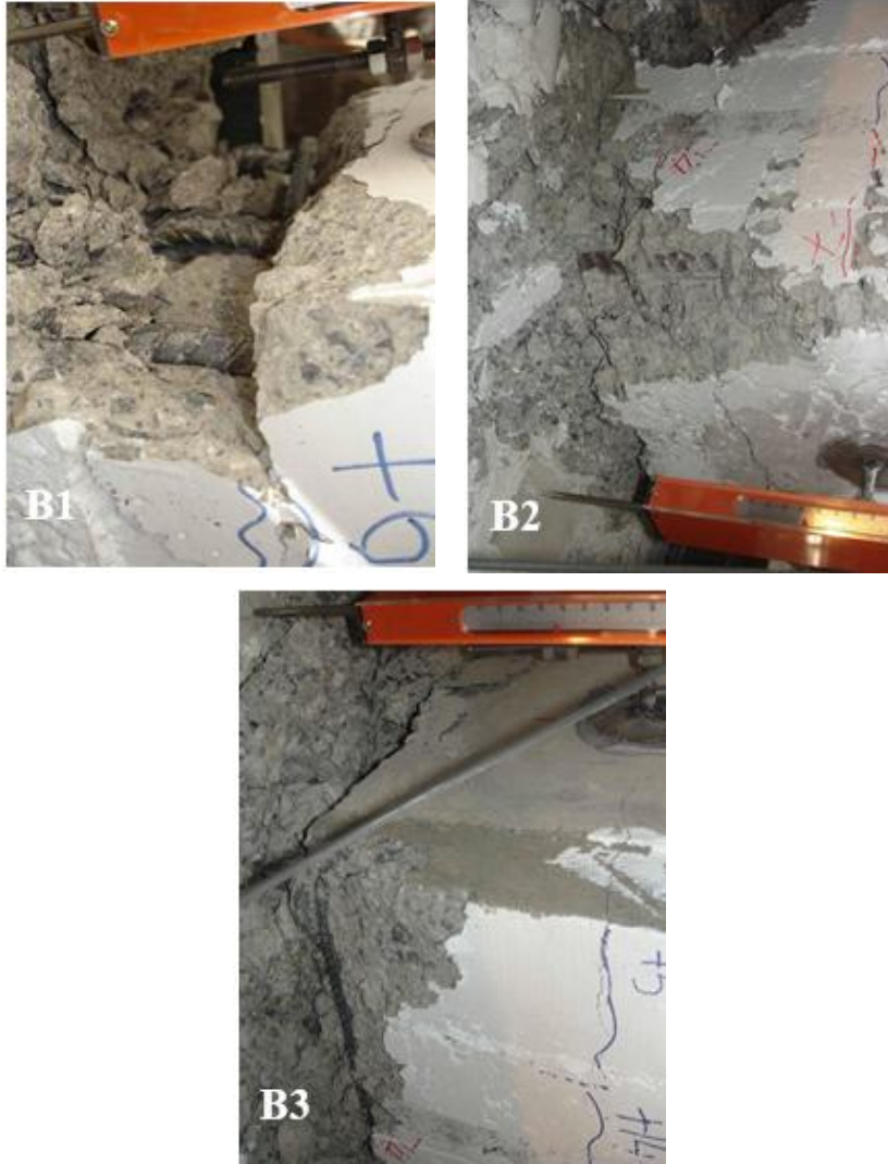
Fig. 4. Restraints damage of specimens (Plastic hinge)
